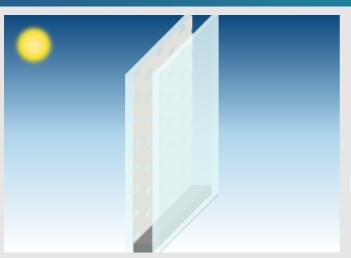
PLANICLEAR (6 mm) BF2WS White (78 %) Design: ID 552 - negative dots Pane 1 Diameter: 1,5mm Cavity 1 ARGON (90%) / AIR (10%) / 16 mm Pane 2 PLANICLEAR (6 mm)
