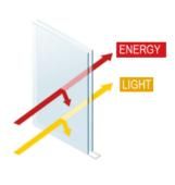
Light and solar radiant heat factors may vary due to the chemical composition of the glass and the production process. These factors refer to test panes as specified by the applicable testing standard. The performance data could deviate absolutely +/- 5 [%]. The Ug-value is calculated without frit. Light and solar radiant heat factors calculated according to EN 410, vertical installation.
