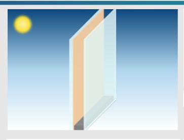
ORAÉ (6 mm) Pane 1 COOL-LITE SKN 183 Cavity 1 ARGON (90%) / AIR (10%) / 16 mm Pane 2 ORAÉ (4 mm)
