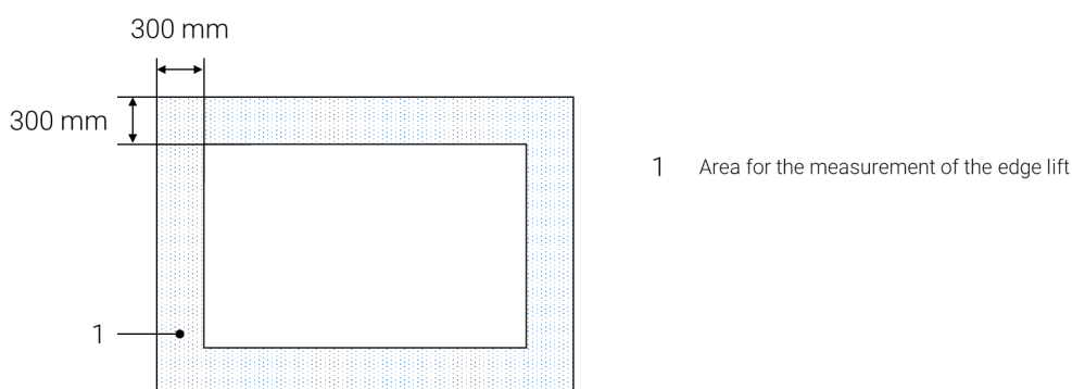
Picture 21: area for the measurement of the edge lift
